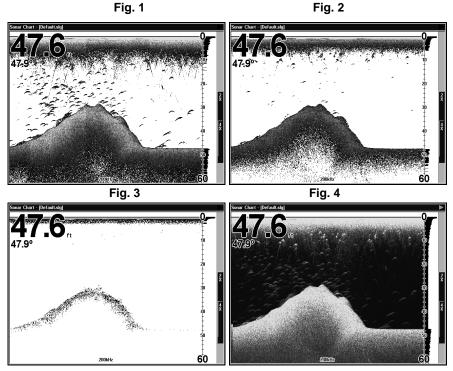
These figures show results of different sensitivity levels on the same location. Fig. 1: Sensitivity at 88 percent. Typical of full auto mode. Fig. 2: Sensitivity set at 75 percent. Fig. 3: Sensitivity set at 50 percent. Fig. 4: Sensitivity set at 100 percent.
